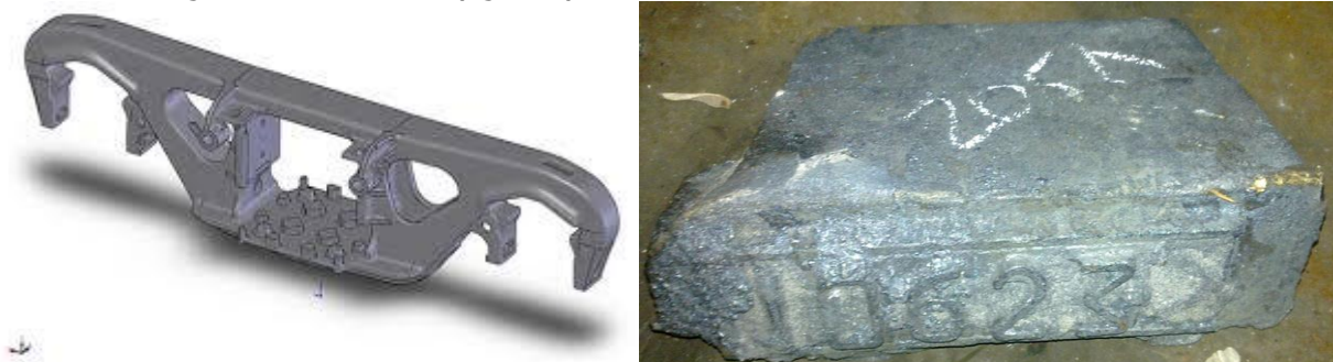
Figure 1-Side frame (a) and process sample (wedge-shaped) (b) of 20GL steel
