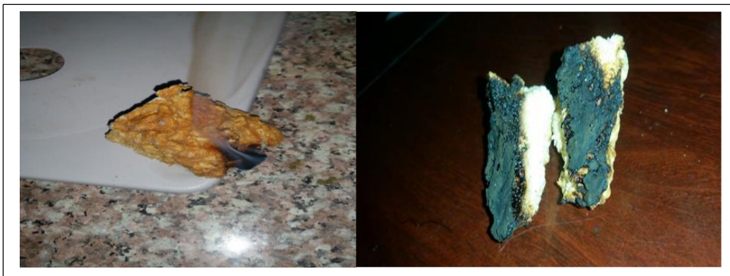
Figure 2: The combustion test of fabricated panels core.
