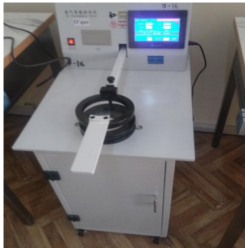
Figure 3. The process of testing air permeability
