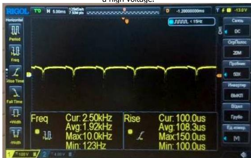
Figure 11. An oscillogram of the input frequency of a KTD718 transistor
