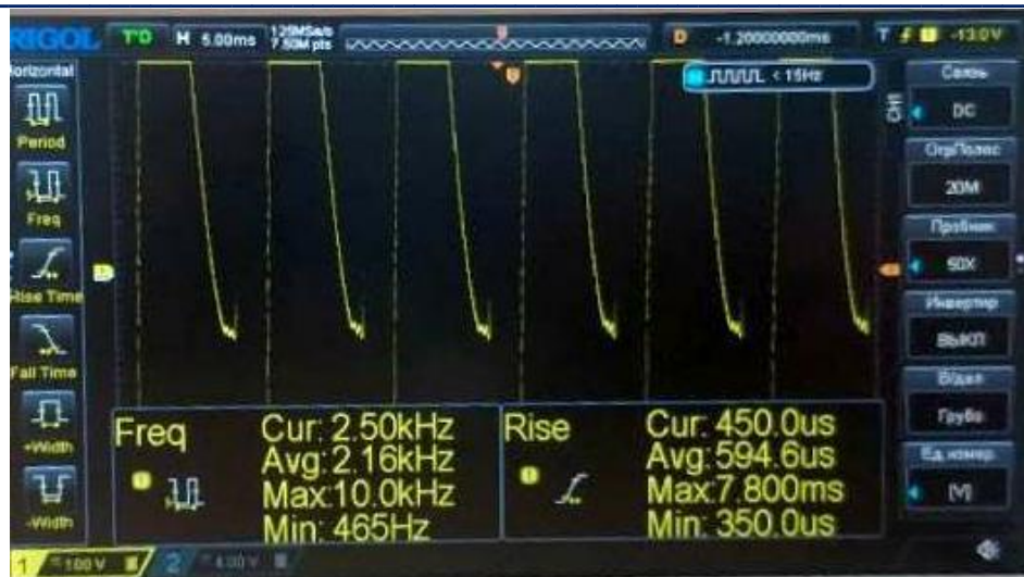
Figure 12. Frequency oscillograms at the output of the transistor KTD718
