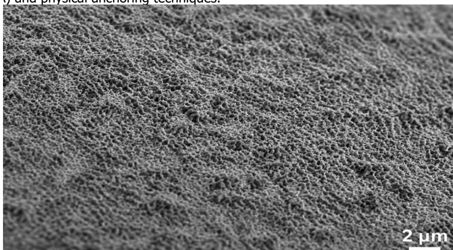
Figure 4. Scanned electron microscopy of textile coating with flame retardant agents.
