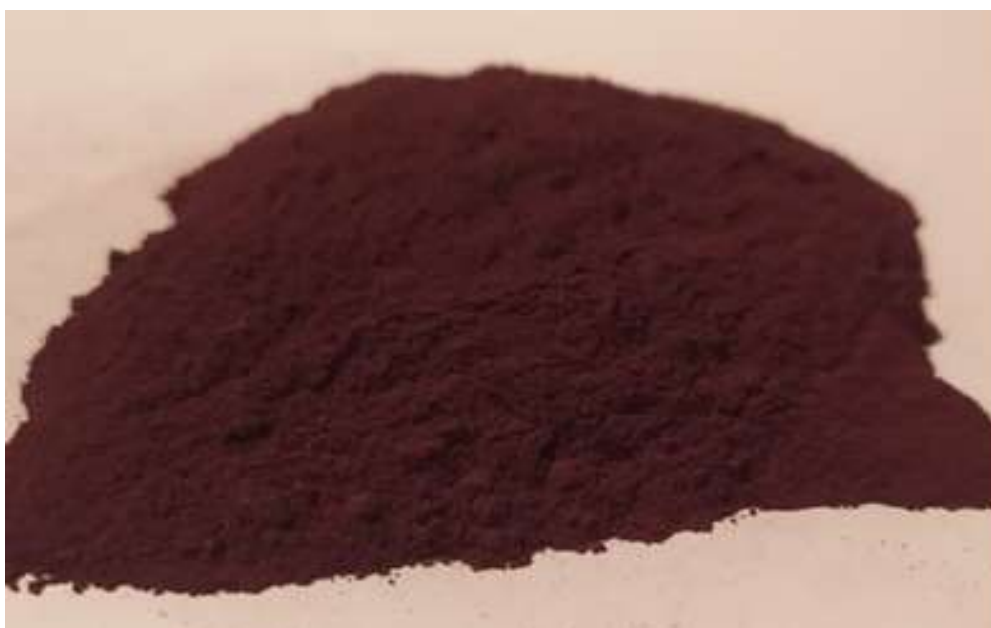
Picture-1. External view of the iron ash (dross) of the Tashkent Metallurgical Plant
