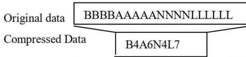
Figure 4: Overview of the run length encoding
