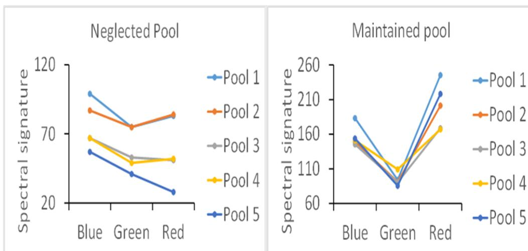
Figure 5: Spectral signatures for both maintained and neglected swimming pools.
