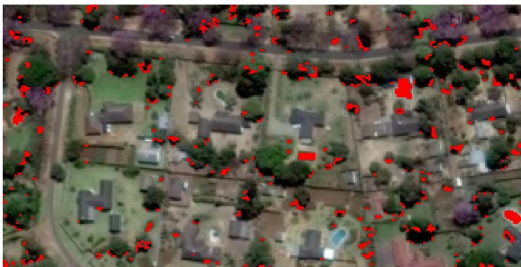
**Figure 8:** Growing feature objects by specifying the area geometry.
