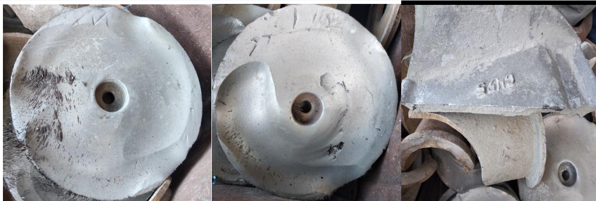
Figure 2. Appearance of a disc cast that has become unusable
