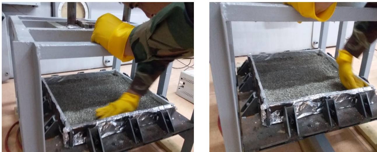
Figure6. The process of obtaining experimental and industrial production batches of vermiculite tile materials.
