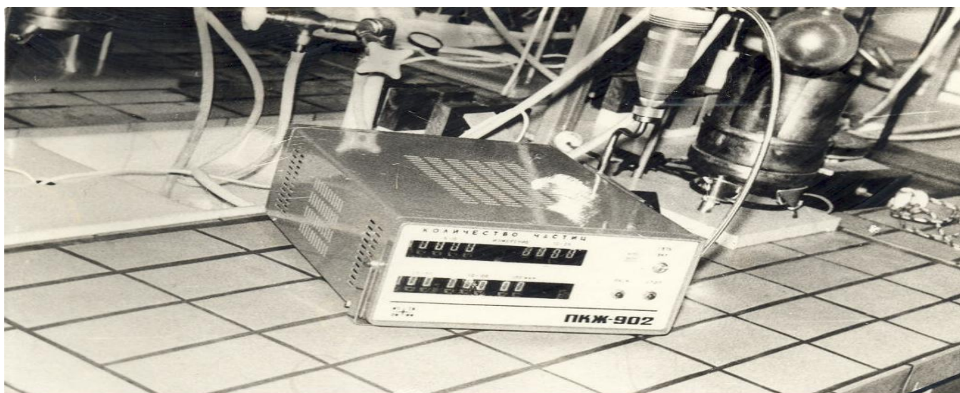
Figure-1. LCD-902 device, designed to detect mechanical particles in the working oil of tractors and combines power transmission devices.
